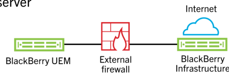
Option 2 - TCP proxy server deployed in the DMZ
