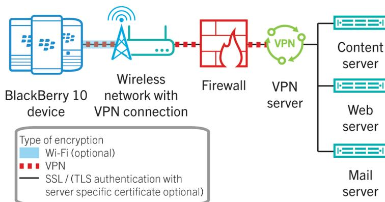
In a VPN connection, devices connect to your organization's resources through any wireless access point or a mobile network, your organization's firewall, and your organization's VPN server. Wi-Fi encryption is used if the wireless access point is set up to use it.
