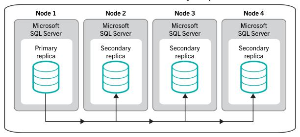
To use an availability group, you configure a WSFC cluster with multiple nodes. Each node is a separate computer that has an instance of Microsoft SQL Server. One of the nodes hosts the primary BlackBerry UEM database and gives the BlackBerry UEM components read-write access. This node is the "primary replica." The WSFC cluster can have one to eight other nodes, each hosting a secondary database. These nodes are "secondary replicas."
