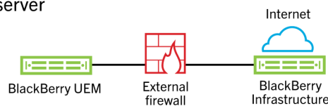
Option 2 - TCP proxy server deployed in the DMZ
