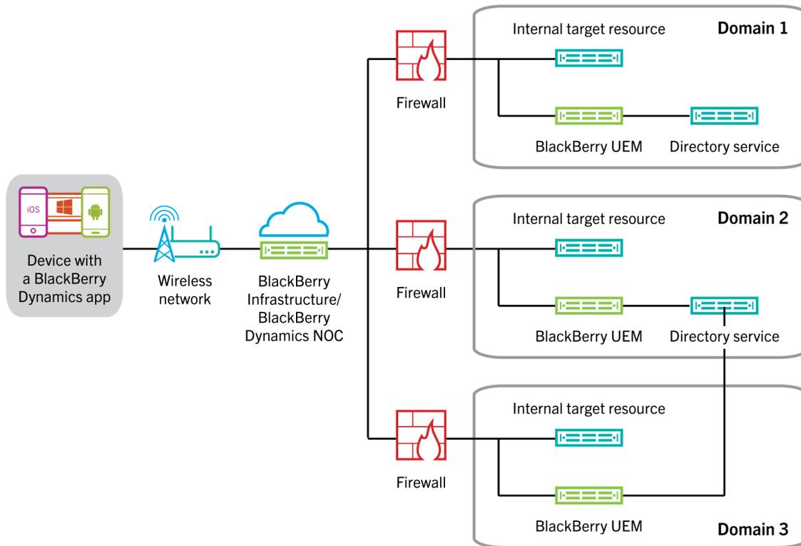
In a multi-realm KCD environment, the BlackBerry Dynamics client selects a BlackBerry UEM Core to process the KCD request based upon the DNS domain of the target server. Once the target is determined to be a KCD target, the BlackBerry Dynamics client determines the list of BlackBerry UEM Core servers that are within the same DNS domain as the target, then randomly selects from this list (based on priorities) a BlackBerry UEM Core to process the request.
