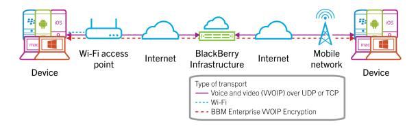
BBM Enterprise video or voice between a device on a Wi-Fi network and a device on a mobile network through the BlackBerry Infrastructure
